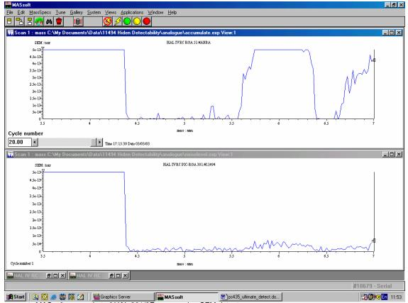
Figure 1: MASsoft screenshot of HAL 301/3F gauge using SEM detector.
