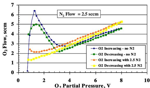
Figure 5a (above). The addition of N<sub>2</sub> flow accelerates target poisoning for AlO<sub>x</sub>N<sub>y</sub>, but can be avoided with two-gas Partial Pressure Control (Figure 5b, below).
