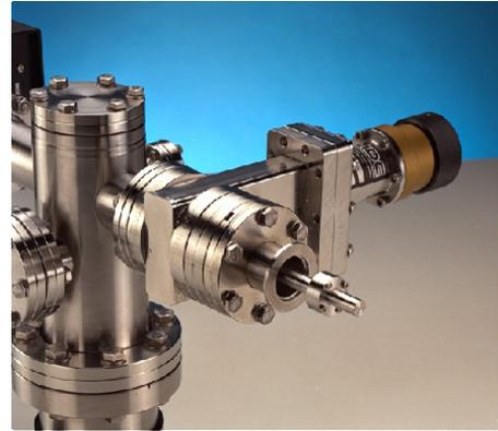
Figure 3. Direct Partial Pressure measurement with the HPR-30 process gas analyser.
