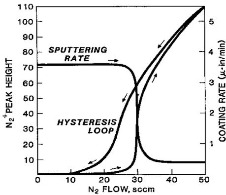
Figure 1. The hysteresis curve for the reactive sputtering of titanium in an argon/nitrogen atmosphere using flow control of the reactive gas.
