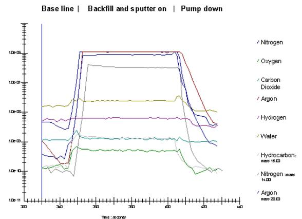
Figure 4a (above) and 4b (below). Auto-switching inlet provides baseline vacuum diagnostics before and after process. The in-process background levels of hydrocarbons and oxygen below are in the ~100ppm range.
