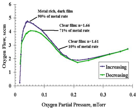
Figure 2. Partial Pressure Control of index of refraction and deposition rate.
